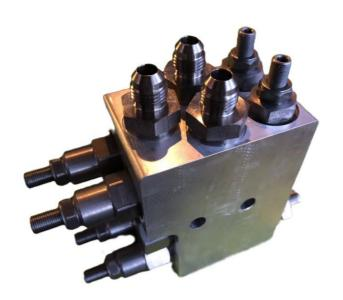
Custom hydraulic manifolds designed for specific applications to minimise pipework, leak paths, overall part count, and cost. Gives significant benefits in reliability and operation.
